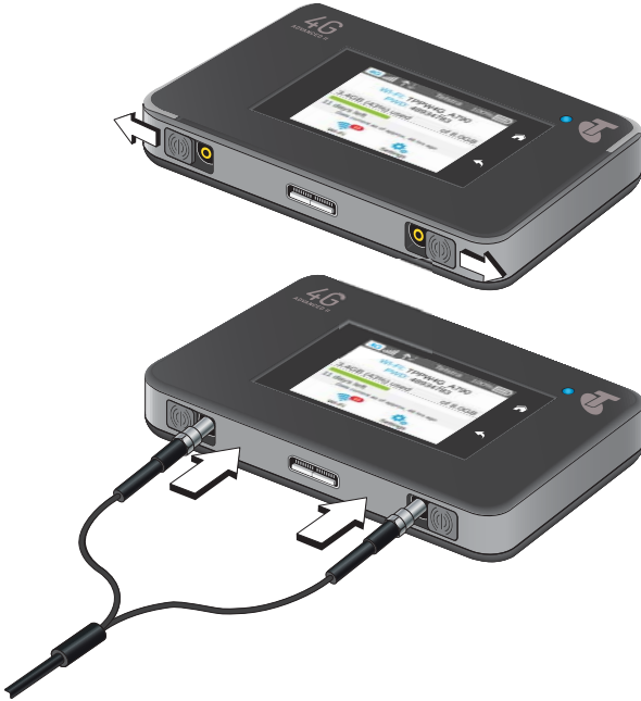
Figure 4. External antennas with TS-9 connectors
