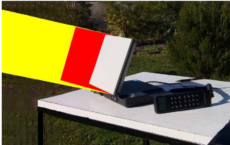
EME Clearance Zone 80cm directly in front of the antenna
