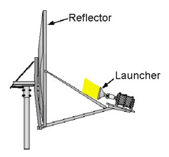
EME Clearance Zone – 30cm from the launcher towards the reflector
