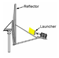
EME Clearance Zone 30cm from the launcher towards the reflector
