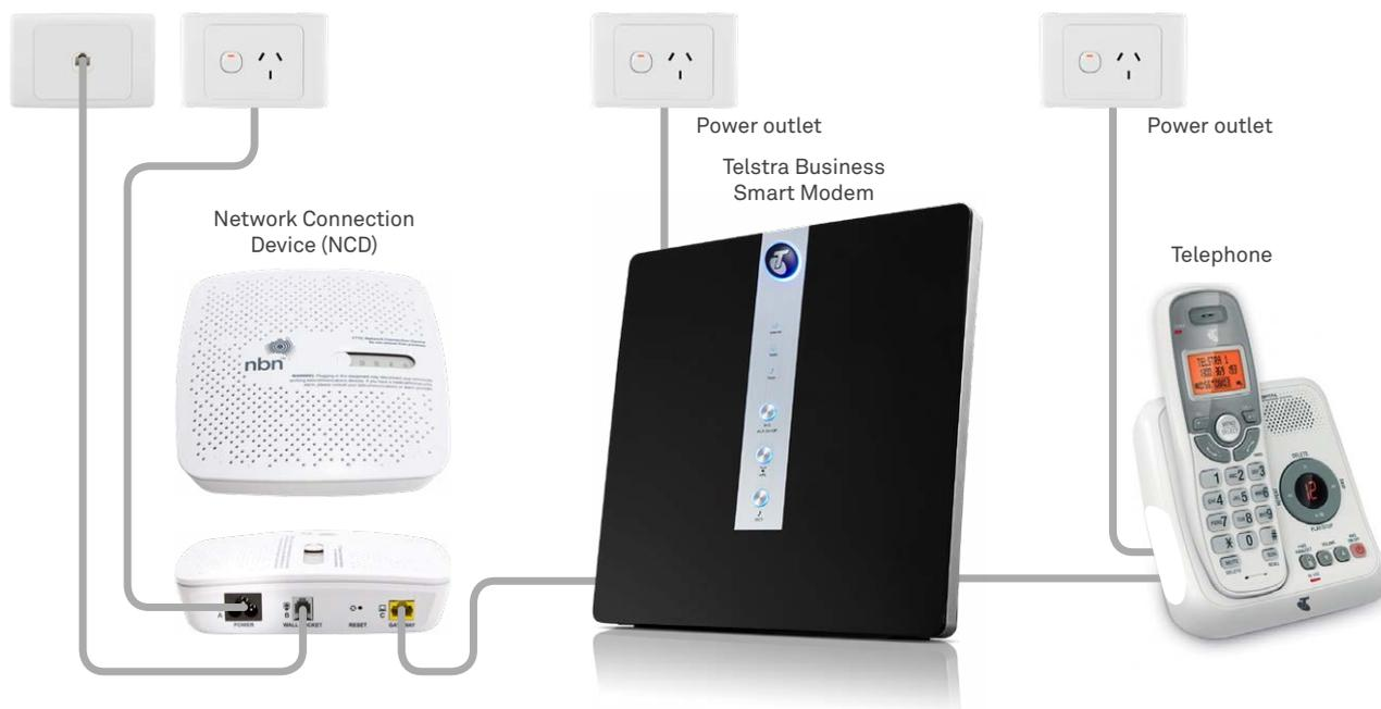
For more information about the nbn equipment and what you need to know, visit [www.nbnco.com.au/learn/network-technology](http://www.nbnco.com.au/learn/network-technology) and view the preparation guide for your connection type - Fibre to the Curb (FTTC)
