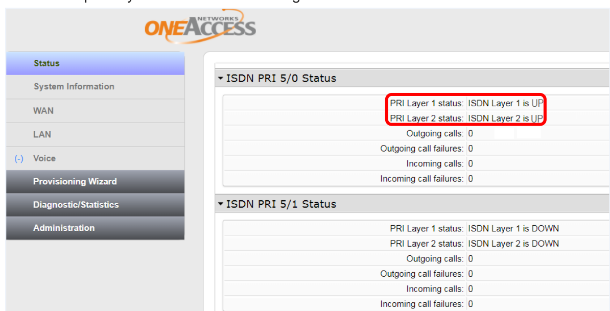
Figure 36: PRA/PRI ports verification
